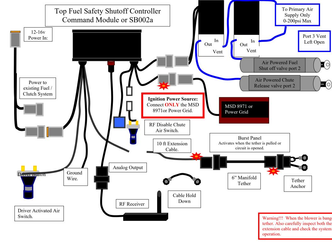
The Electrimotion Safety Shutoff box is designed to shut the car off as a result of a catastrophic event. The box has 3 trigger inputs (sb002), 5 inputs (Command Module) which will trigger 3 separate output events. The 3 trigger inputs are a burst panel input, an air activated driver push button trigger input and a wireless shut down input, CM has pan psi input and wheel counter inputs as well. The Command Module also has, a throttle release output.
