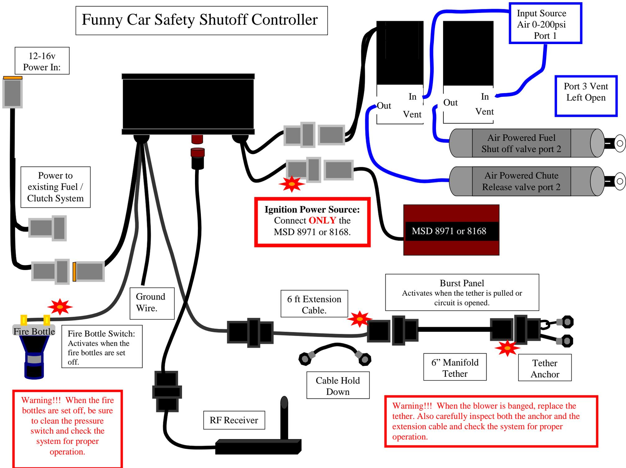
The Electrimotion Safety Shutoff box is designed to shut off the car as a result of a catastrophic event. The box has 3 trigger inputs, which will trigger 3 separate output events. The 3 trigger inputs are a burst panel input; a Fire Bottle trigger input and a wireless shut down input.
