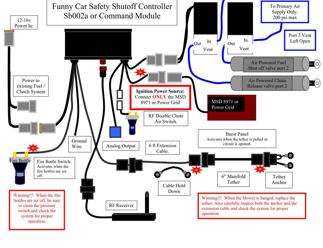
The Electrimotion Safety Shutoff box is designed to shut off the car as a result of a catastrophic event. The box has 3 trigger inputs (sb002a) or 5 inputs (Command Module), which will trigger 3 separate output events. The 3 trigger inputs are a burst panel input; a Fire Bottle trigger input and a wireless shut down input. The Command Module also has, a throttle release output.
