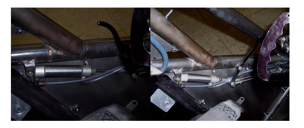
Typical Mounting of Fire Bottle Air Switch.
