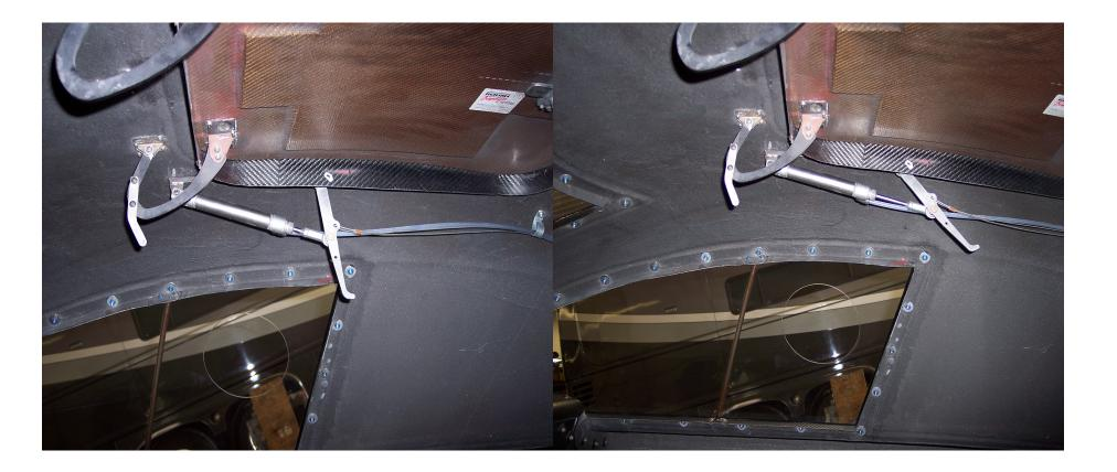
Typical Mounting of Fire Bottle Air Switch.
